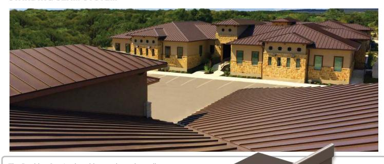
The Berridge Cee-Lock architectural metal standing seam panel is designed for residential or commercial construction over solid sheathing. This 1½" high panel incorporates an integral snap-lock seam and an optional extruded vinyl weatherseal. The standard coverage option is 16½" and its optional 11½" coverage adds versatility.
